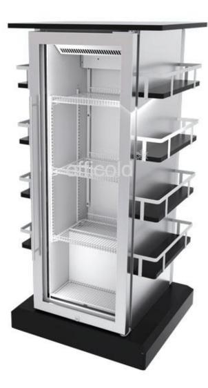
External dimensions (mm) 565 x 540 x 1180 Net weight (kg) 75 Internal net volume (Lt) 85 Capacity cans 33cl / pet 500ml (pcs) 96 / 44 Door serigraphy dimensions (mm) 306 x 958 Transport 40' container / 13m truck 76 / 92 24h energy consumption (kW/h) 1,88 Climatic class CC2-K4 (32°C/65%HR) Temperature range (°C) 0 / +6,6 Refrigerant R-600a Voltage / frequency 230v / 50Hz Sound level (dBa) <40
